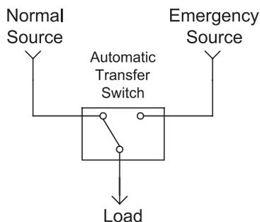
**Figure 10-2: Automatic transfer switch one-line diagram representation**
