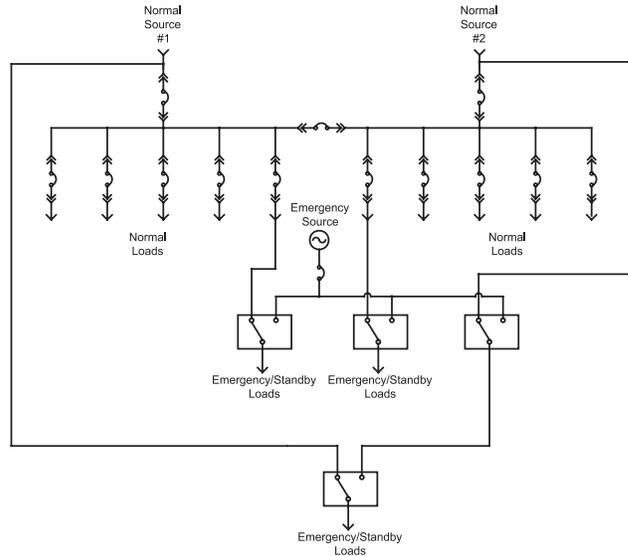
**Figure 10-5: Example of a more complex emergency/standby system arrangement**
