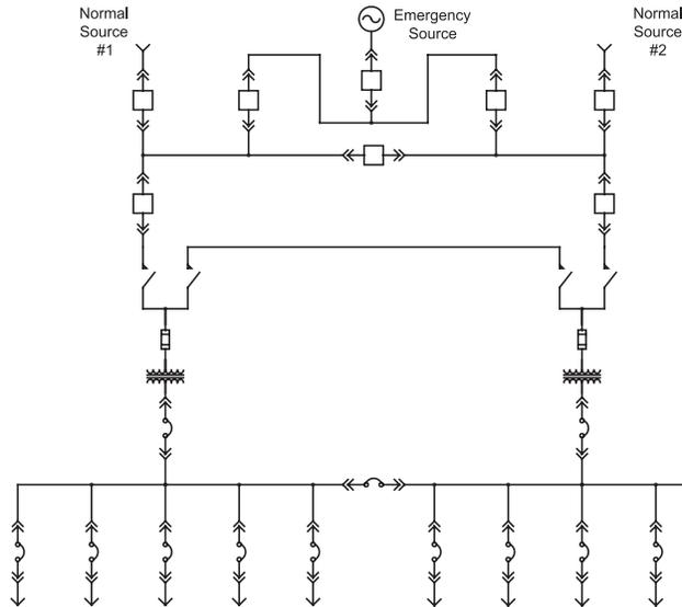
**Figure 10-6: Medium voltage emergency/standby system implementation**
