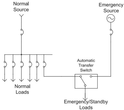
**Figure 10-4: Simple emergency/standby system arrangement**
