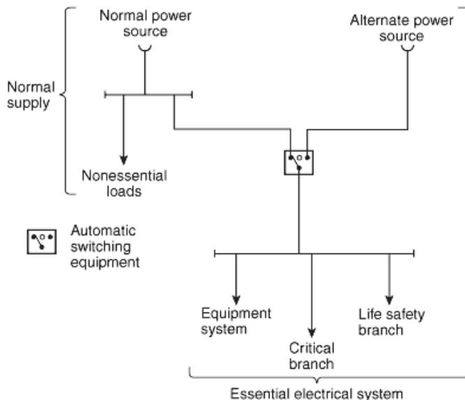
**Figure 10-7: Minimum requirement per NEC [2] and NFPA 99 [5] for essential electrical system for hospitals 150 kVA or Less (same as [2] FPN figure 517.30 No.2)**
