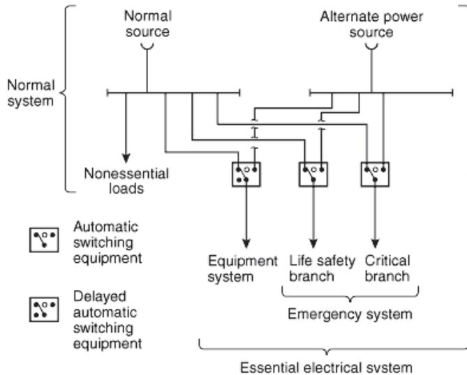
**Figure 10-7: Minimum Requirement per NEC [2] and NFPA 99 [5] for Essential Electrical system for Hospitals over 150 kVA (same as [2] FNP figure 517.30 No. 1)**
