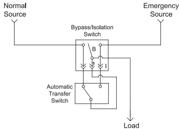
**Figure 10-3: Bypass/isolation switch application**
